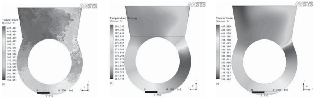
Picture 8 – Temperature distribution in the channel furnace. Left: intermediate distribution after 45 sec (LES), middle: time averaged over 60 sec (LES), right: steady-state (k-ε model)
