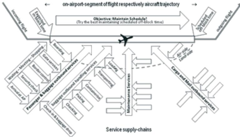
Figure 2 – High-level Model with Exemplary Ground Services
