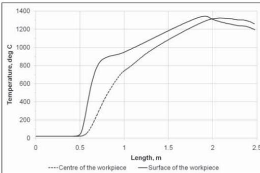
Figure 4 – Temperature distribution along the workpiece during the first start of the heater
