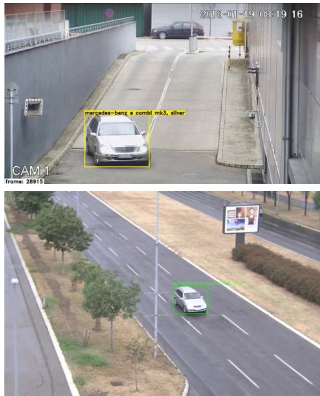
Fig. 5.22. Scenario with detecting re-identifying a vehicle in aerial image. The vehicle has been first classified for make-model-sub model-year and color labels in the scene presented in the top part of the figure, captured by a fixed camera. The same vehicle re-appeared in the aerial image in the bottom part of the figure and was positively re-identified as silver-colored Mercedes E Combi MK3 sub model.
