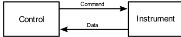
Fig. 11.1. Illustration of the VISA standard overseeing the communications between a control unit (e.g., a computer) and an instrument, connected with any type of interfaces supported by VISA.
