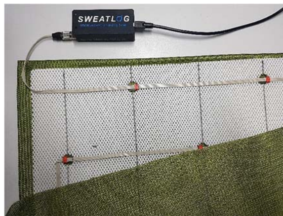
Fig. 6.7. SWEATLOG logger and sensor array (mat) with up to 60 HIH8xxx sensors at one I2C ribbon (4 wires).
