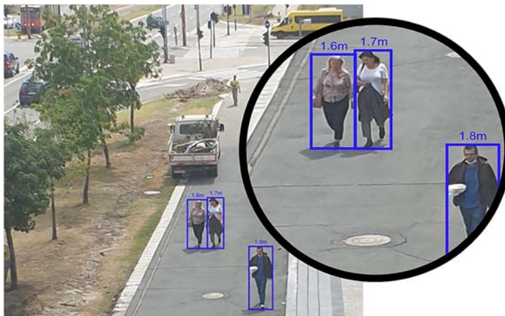
Fig. 5.19. People detected on a sidewalk using a drone camera. Enlarged view of pedestrians with estimated heights enlarged in the framed circle in the left.
