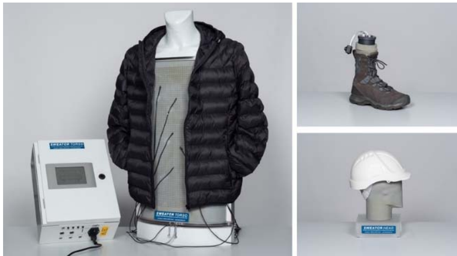
Fig. 6.9. SWEATOR torso with test jacket, SWEATOR foot and SWEATOR head with safety helmet.
